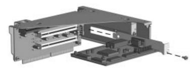
Removing the Expansion Board
