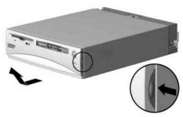
Removing the System Unit Cover
